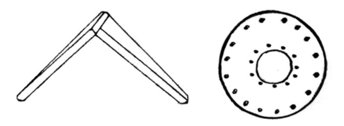
A **lens shield**, shown on the left, is attached above the lens hole. On the right is a **compact disc** with nails on the inner and outer rim; this is fitted over the lens hole.
